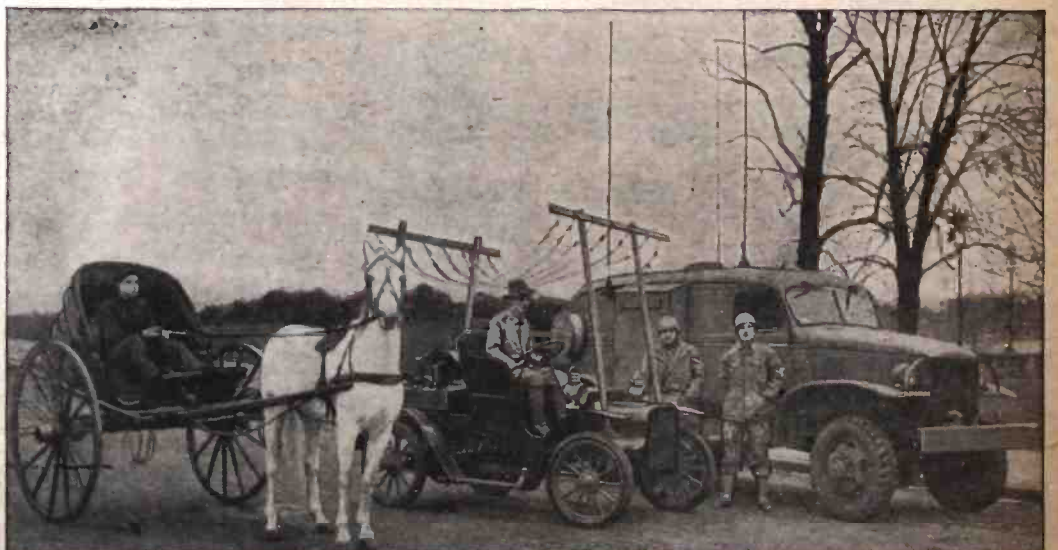
The two-wheeled telegraph cart dates back to 1863. It was succeeded in 1907 by a 1-cylinder Cadillac. The modern unit (right) is a complete mobile station, Hallicrafters SCR-299.
